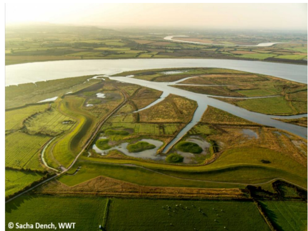
Above: restoration of wetlands provide effective flood management, with wetlands acting as natural 'sponges' to soak up flood waters. Image from Somerset, UK.
