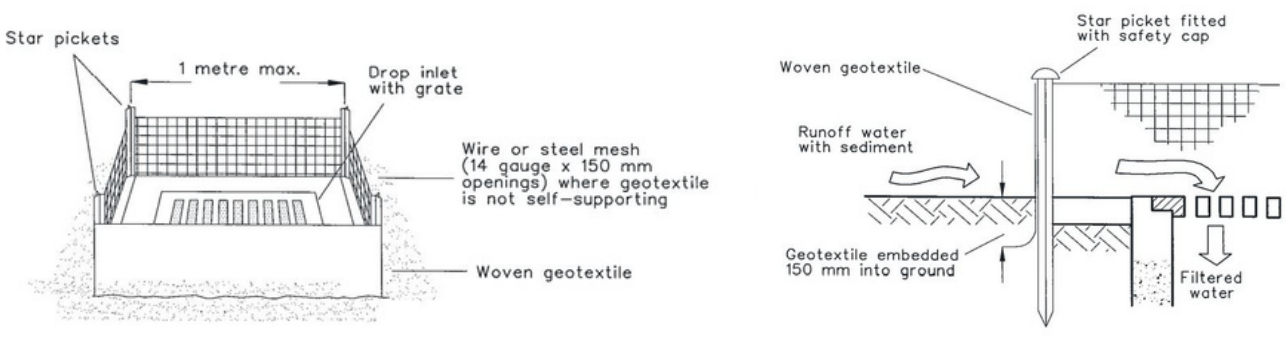
Figure 18: Construction details of a sediment fence for stormwater pit protection. Figure from Landcom 2004 'Soils & Construction Volume 1 Managing Urban Stormwater (4th edition)'.
