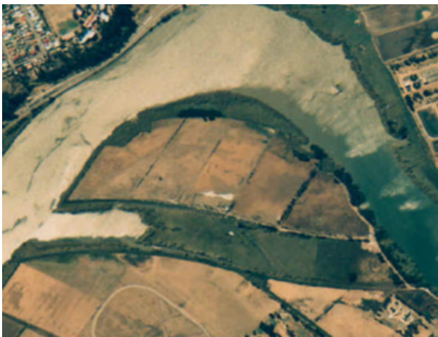
Above: satellite imagery shows Hunter's Cut, a failed attempt to straighten the estuary.
