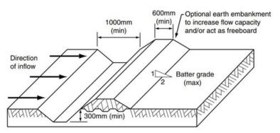
1. Diversion drain. The drain channel must be at least 150 mm deep with a curved shape that will be site specific. Stabilise the flow path to protect it from scour by lining the drain with matting or rock. If dispersive soils are present, create diversion drains by building soil berms instead of digging.
