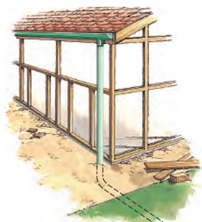
Figure 6: It is important to connect downpipes as soon as impervious surfaces are created. Figure modified from the 'Do It Right On Site' brochure series, Southern Sydney Regional Organisation of Councils.
